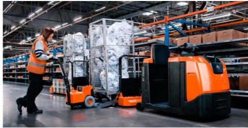
The BT Movit model TWE080N is a low-cost compact version which is shorter, and features a differential gearbox giving a tight turning circle. This model is also lightweight making it easy to handle.
