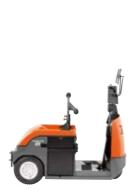
Compact 4CBTY models are available with capacities of 2 and 4 tonnes – ideal for work in confined areas with a width of just 800mm
