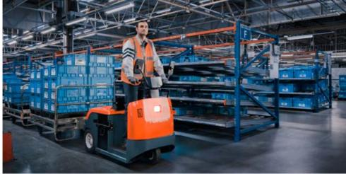
Pneumatic tyres mean smooth driving on uneven surfaces, to aid operator comfort. The compact design of Toyota Tracto S-series models allows them to work efficiently in confined spaces, and the narrow chassis width is ideally suited to driving in narrow traffic lanes where multiple load movements are taking place.
