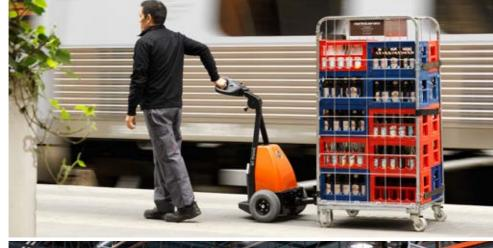
These pedestrian-operated units can be used as part of an integrated handling process, to take care of heavy load movement.
